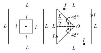
Let a current, I pass through the square loop of side, L. The magnetic field at the centre O,
