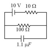
At the steady state, there will be no current through the capacitor. Therefore, potential difference across capacitor  $V_c = \left(\frac{10}{110}\right) \times 100 \; \mathrm{V}$ .
